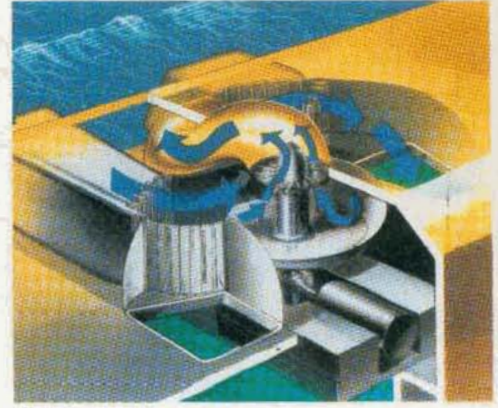
The turbine is directly coupled to an electric generator which is normally housed behind the front chambers in the main body of the converter.
