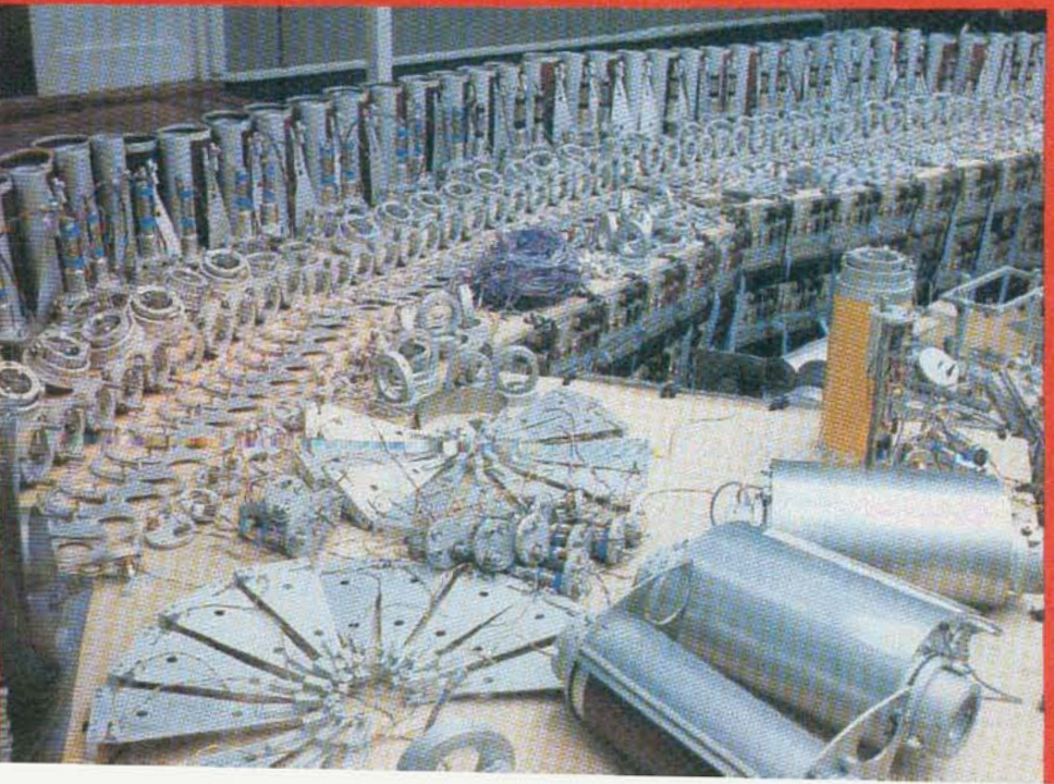
Above The wave power generator Kaime in open sea tests in August 1979. The tests are part of a joint research project by the International Energy Agency, involving Eire, Canada, Japan, the UK and USA in wave power research. The key components are air turbines comprising blades fitted to aluminium and bronze discs. Water under the ship acts as a piston and valves allow air to flow through the turbines in one direction only.
