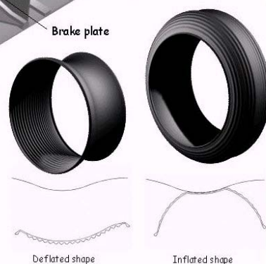
Figure 3: Membrane inflated and deflated shape
