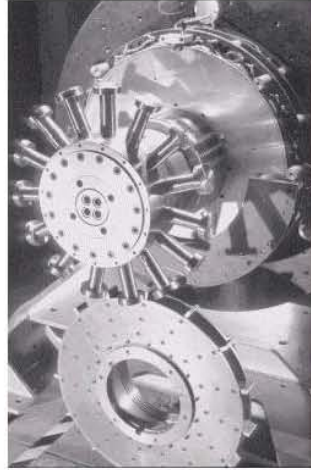
Photograph 1 (right) Partly assembled turbine. Pitching plate assembly on floor; one set of coils has been removed to reveal aluminium eddy current disc.
