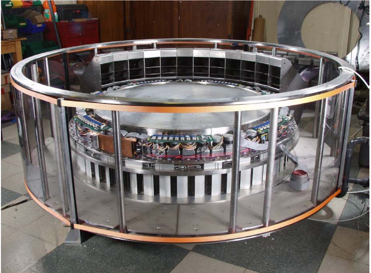
Photo 1: Flow table drained and with the nearer bends removed, showing the rotor foils, stepper-motors and electronics boards
