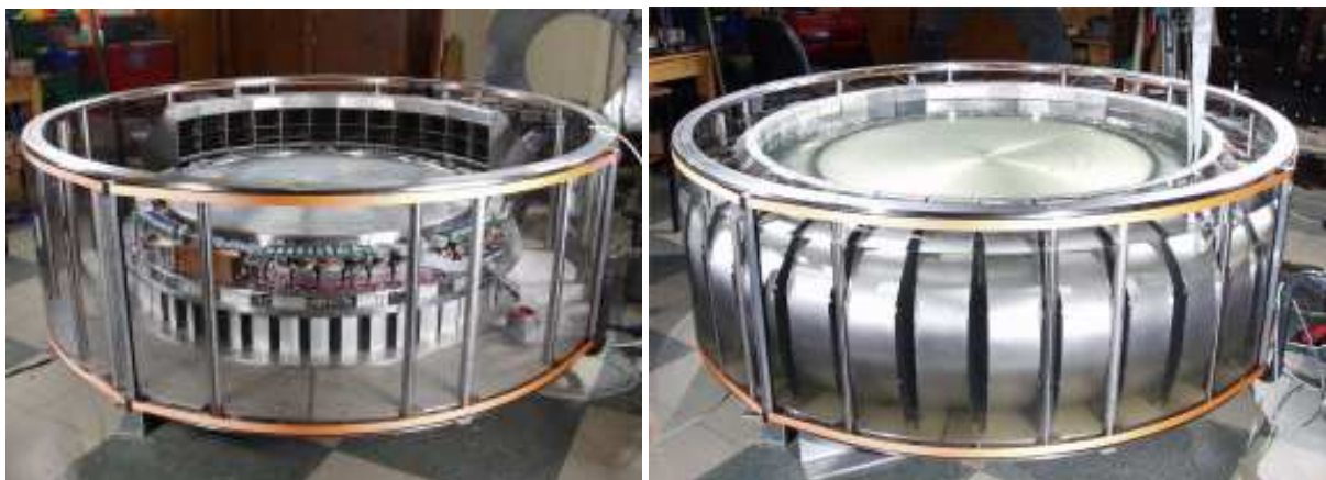
Figures 19 & 20: The flow table. The EPSRC financed and recently completed flow table demonstrates the flow generation concept proposed for the circular tank and provides a useful test facility for small scale tidal stream research. The foils of the vertical axis rotor are visible in the dry and unclothed view at left. Above the foils is a ring of 56 stepper motors which are computer commanded to set the shape of a deformable multi-lobe cam band. Individual foils track the cam profile so as to cyclically vary pitch and thus either push or pull water into or out of the test region above. Twelve flow re-directing bend units can be seen at the back. In the operational wet view at right the complete ring of 36 bends is in place.
