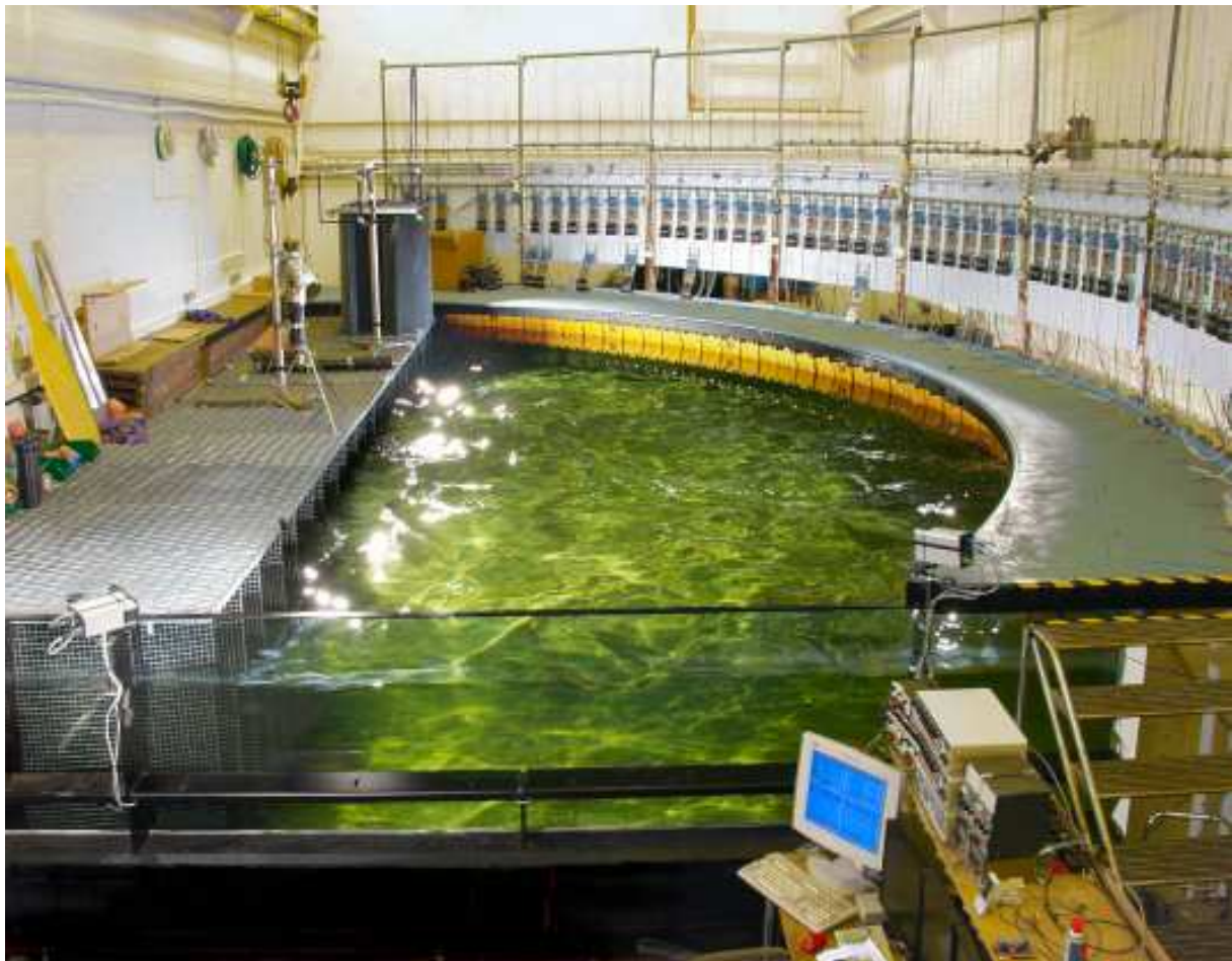
Figure 1: The Edinburgh curved tank. The sea-state is a one second Pierson-Moskowitz with cosine spreading. The top bars of the open tubular structure at the back of the curved platform support the ends of springs that pull the wavemakers back to the centre of their working range against the hydrostatic pressure on their front faces. The paddles look static because the image is a composite of 12 photographs.
