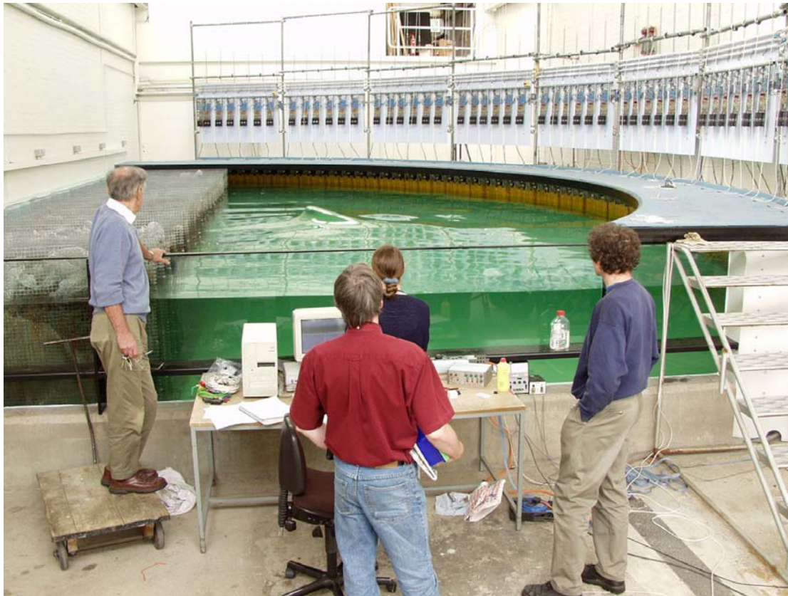
Figure 2. The generation of a freak wave is a good way to check the tank transfer function.
